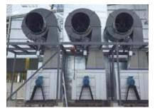
**CENTRIKLON** The high capacity CDS Centriklon centrifugal separator removes dust and chaff even more efficiently than the CAC system. No moving parts means minimal maintenance.
