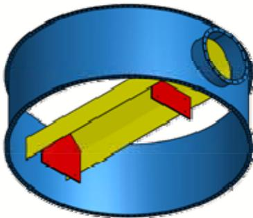
The SimPact® 4T-R construction form 17 and 17 WB have radial filter inlet with an integrated diffuser system, introducing the airflow below the filter bags.
