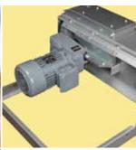
Direct-mounted gearbox motor with support frame.
