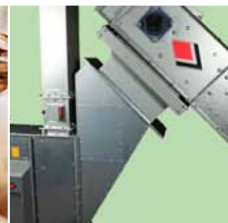
Connection hopper between conveyor and elevator.
