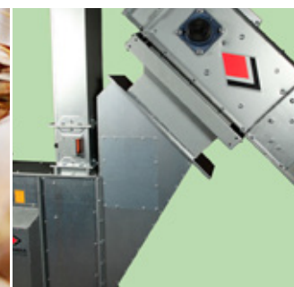
Connection hopper between conveyor and elevator.
